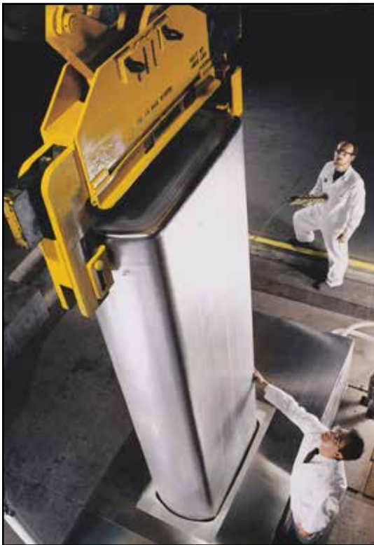
Erach Tarapore (lower right) and Jeff Dickinson (upper right) with an aluminum casting, which utilized electromagnetic casting technology that improved product quality. This particular casting made aluminum beverage cans.
