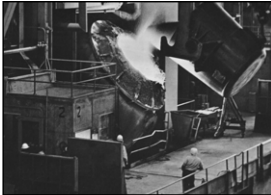
Kaiser engineers developed a method of making steel in minutes instead of hours as soon here at the Fontana, CA, plant.
